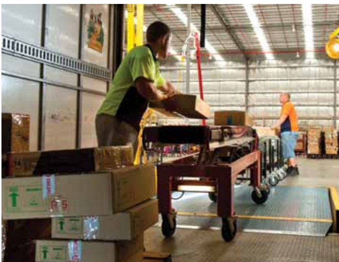
Left: Thomas Collyer (left) and Tom Bowen using the new carton conveyor system at the Erskine Park storage facility in New South Wales.
