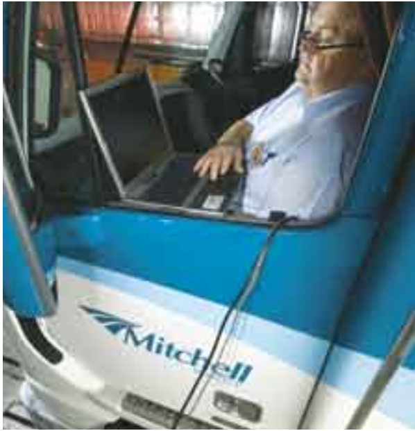
Technical Coordinator Peter Armstrong carrying out diagnostic tests on an LNG-converted prime mover at Kewdale, Western Australia.
