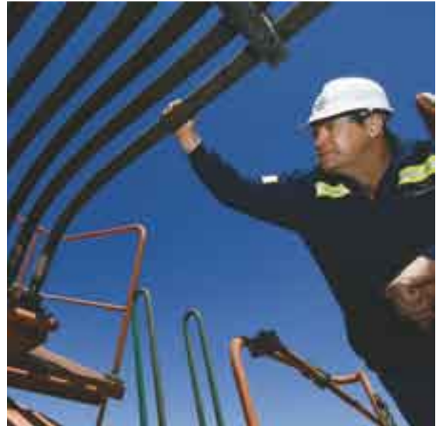
Fitter Bill Clazie checking hoses on an excavator as part of the hydrocarbon management programme.
