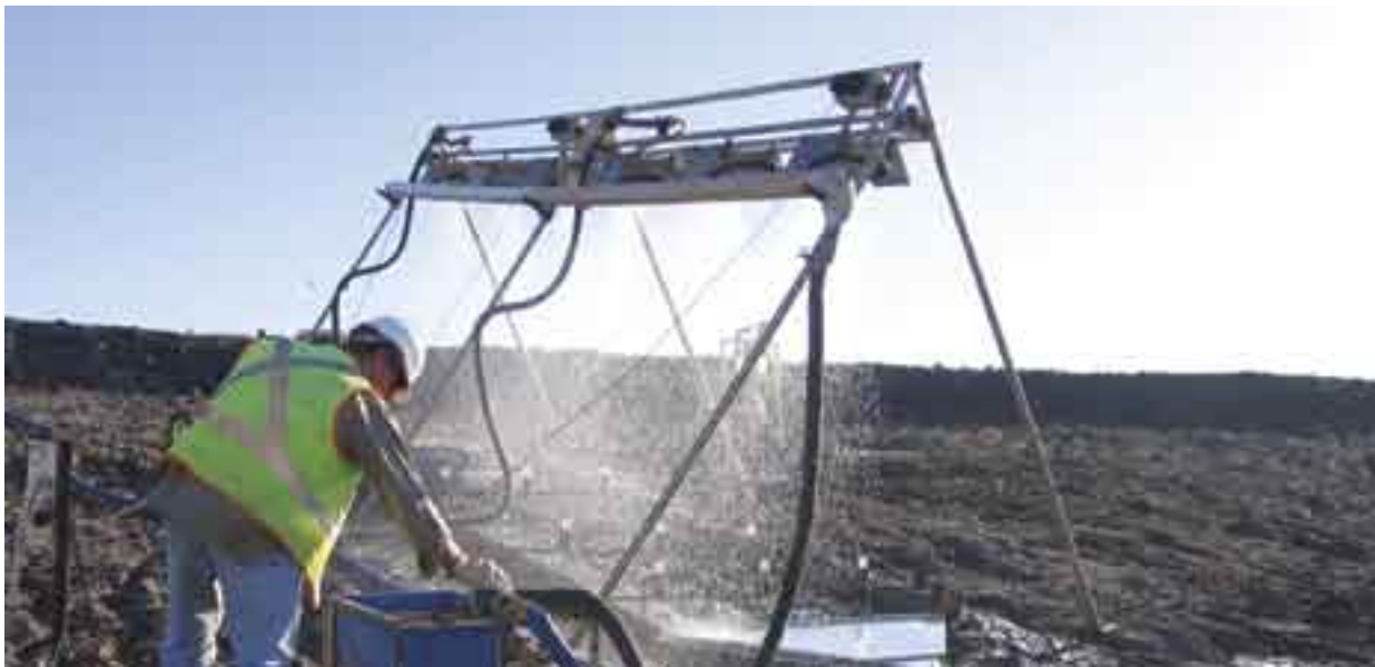
Rainfall simulation to improve dump designs and the rehabilitation prescription.
