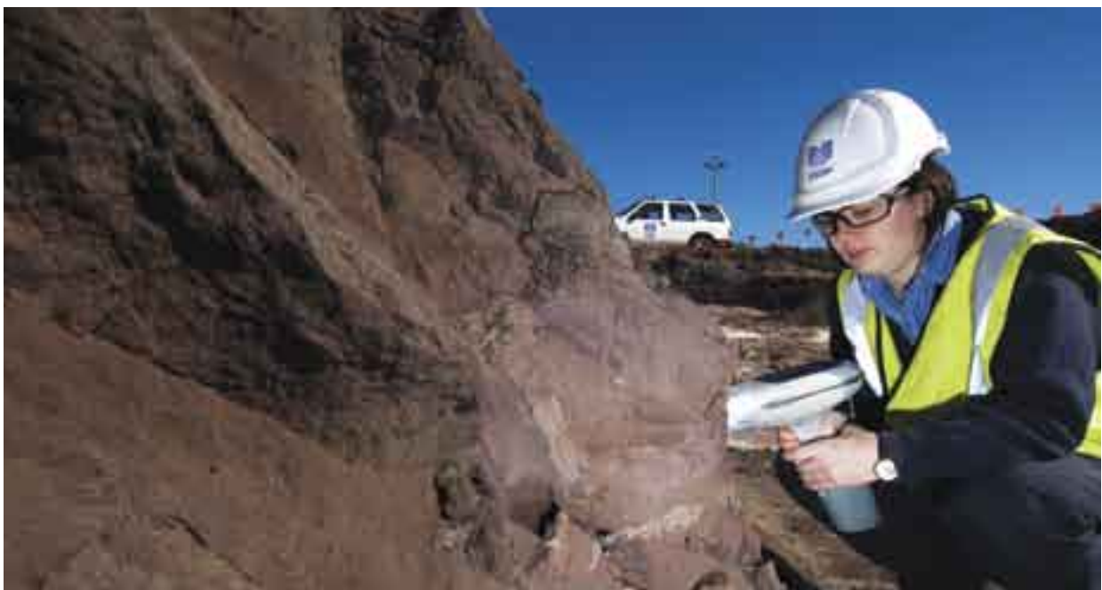
Environmental Advisor Laurinda Shaw taking soil readings during remediation work at the Bayswater site.
