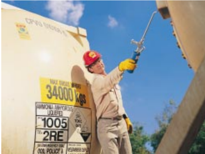
Left Operator Stuart Wragg gas testing for leaks on isotainers at the ammonia rail loading facility.
