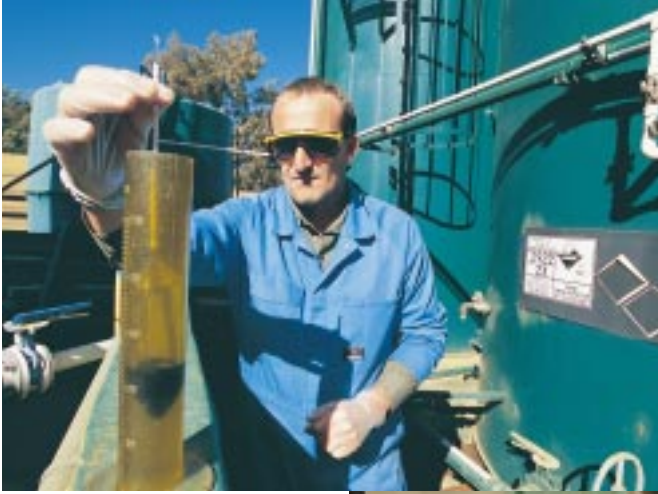
Left Operator Karl Sykes taking a hydrometer reading at Mundijong.
