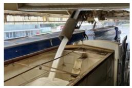
Best reliability: Additional solids load out capacity in Esperance has increased solids despatch capacity by 75%
