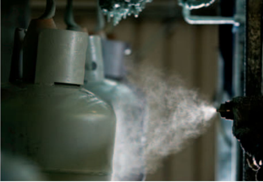
Paint spraying on a Kwikgas 8.5kg cylinder in the automated spraybooth at the Kwinana Gas Terminal in Western Australia.
