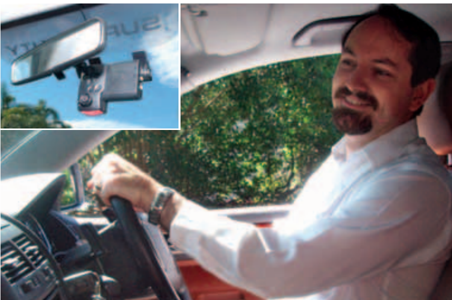
DriveCam in action. The recorder sits behind the rear vision mirror and logs driver behaviour.
