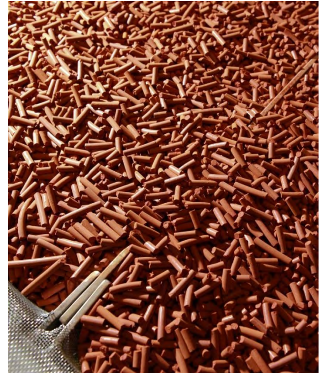
Catalyst to reduce nitrous oxide emissions at CSBP Kwinana
