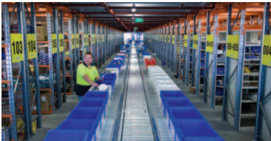
Blackwoods Storeman Darren Carles in the Carole Park warehouse in Queensland using a specially-designed conveyor system to reduce manual handling.
