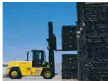
**Forklift operator stacking strip lifts of sawn jarrah at Welshpool.**
