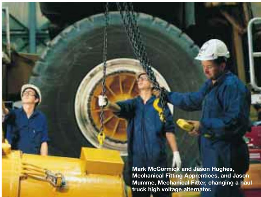
**Mark McCormick and Jason Hughes, Mechanical Fitting Apprentices, and Jason Mumme, Mechanical Fitter, changing a haul truck high voltage alternator.**
