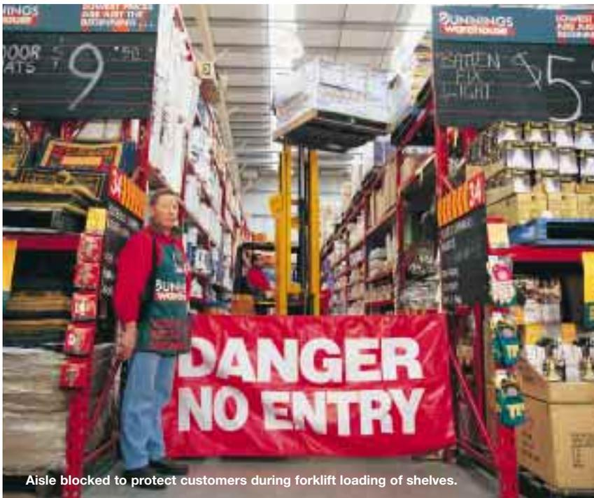
Aisle blocked to protect customers during forklift loading of shelves.
