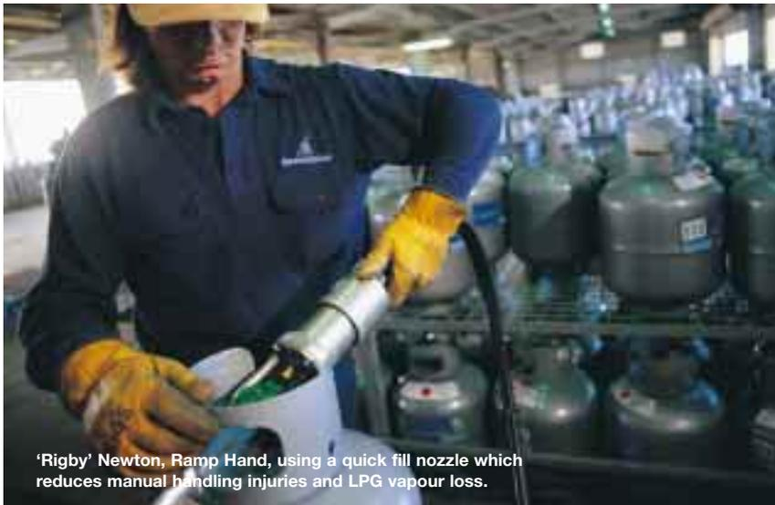
'Rigby' Newton, Ramp Hand, using a quick fill nozzle which reduces manual handling injuries and LPG vapour loss.
